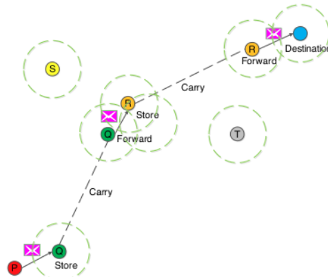
Figure 1. Store-carry-forward mechanism on DTN
