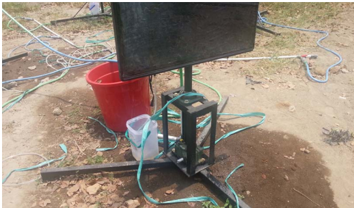
Fig. 2. The Vertical Solar Still with Gearbox to ease rotating the Basin
