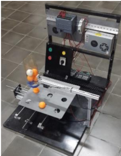
Figure 6. Object Placement System Based on Siemens S7-1200
