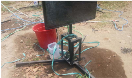
Fig. 2. The Vertical Solar Still with Gearbox to ease rotating the Basin
