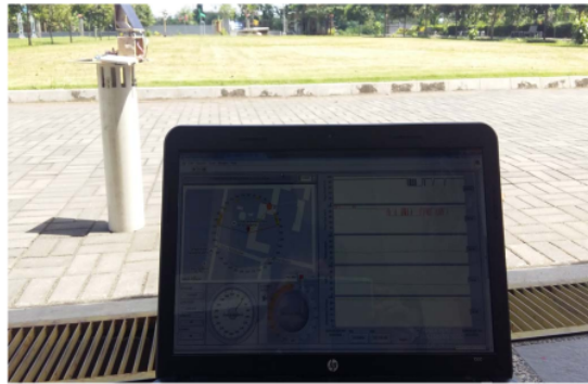
Fig. 5. Control and monitoring whole system from computer wirelessly using LabVIEW software and Bluetooth communication
