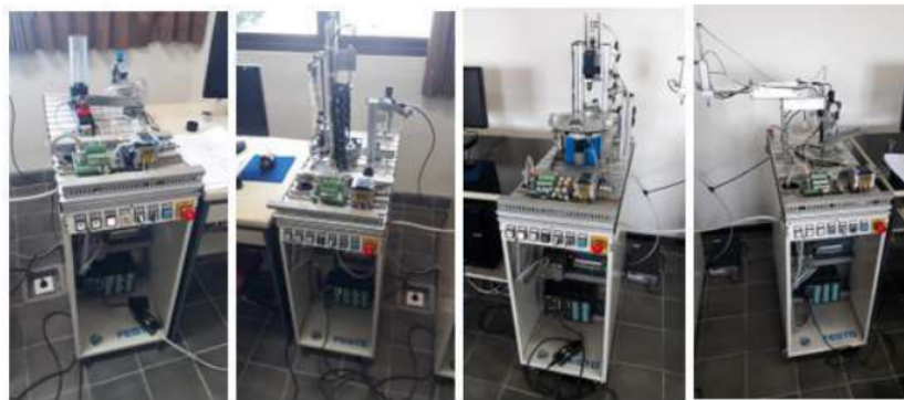
Figure 4. Modular Production System (MPS), a=Distibution Station, b=Testing Station, c=Processing Station, d=Handling Station.
