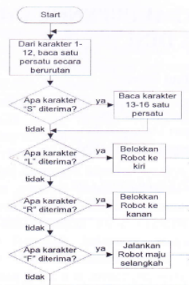
Gambar 13. Flowchart program Robot Beroda
