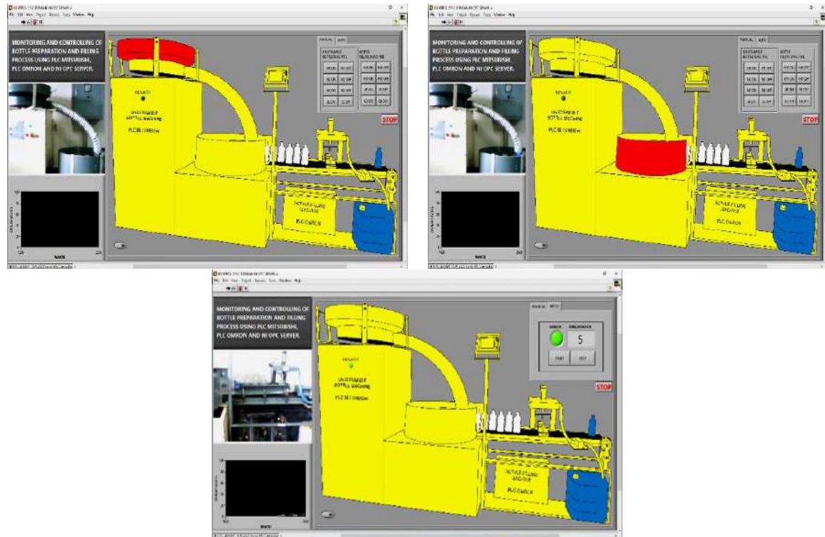
Figure 13. The result of display in LabVIEW according to the actual physical conditions on the field application
