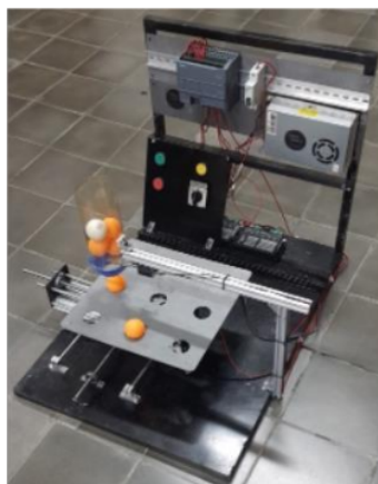
Figure 6. Object Placement System Based on Siemens S7-1200
