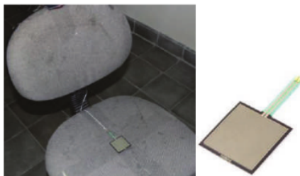
Fig. 2. A FSR sensor is placed on top of the seat cushion
