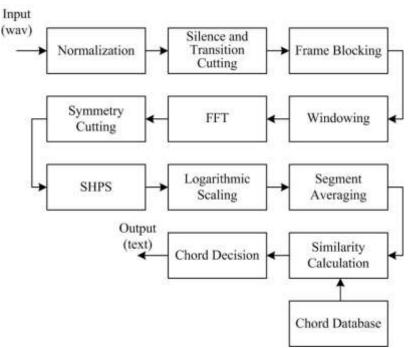
Figure 1. The block diagram of the developed chord recognition system.
