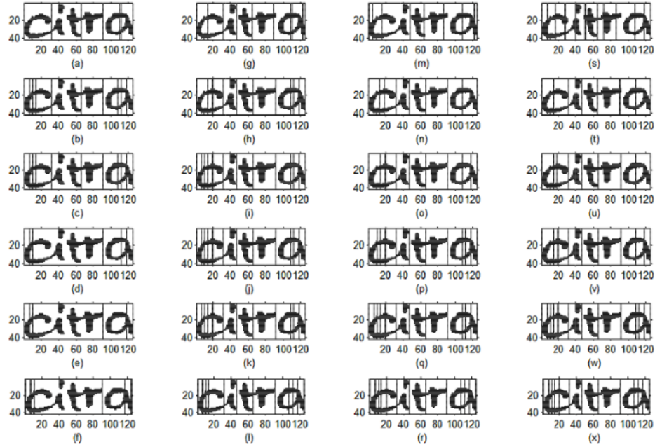
Fig. 6. Segmentation results on various parameters of Kaiser window: (a) – (f) Length: 4 points, \beta values: 0, 10, 20, 40, 80, and 160 respectively; (g) – (l) Length: 8 points, \beta values: 0, 10, 20, 40, 80, and 160 respectively; (m) – (r) Length: 12 points, \beta values: 0, 10, 20, 40, 80, and 160 respectively; (s) – (x) Length: 16 points, \beta values: 0, 10, 20, 40, 80, and 160 respectively. (Notes: Vertical and horizontal axes units are in pixels)
