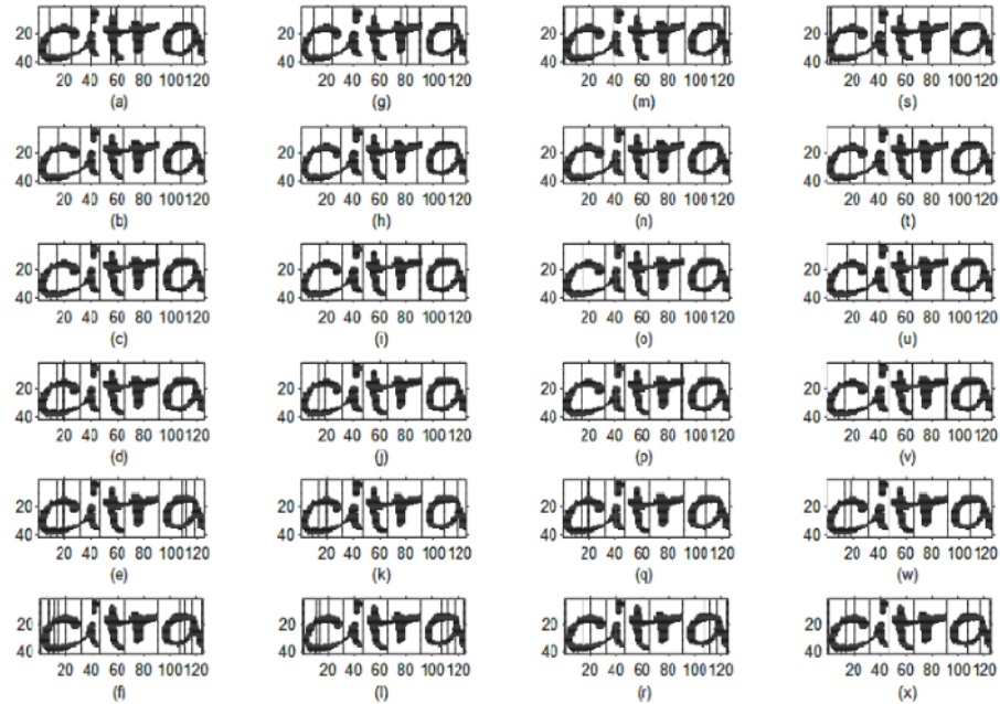
Fig. 7. The Segmentation results on various parameters of Kaiser window; (a) – (f) Length: 20 points, \beta values: 0, 10, 20, 40, 80, and 160 respectively; (g) – (l) Length: 24 points, \beta values: 0, 10, 20, 40, 80, and 160 respectively; (m) – (r) Length: 28 points, \beta values: 0, 10, 20, 40, 80, and 160 respectively; (s) – (x) Length: 32 points, \beta values: 0, 10, 20, 40, 80, and 160 respectively. (Notes: Vertical and horizontal axes units are in pixels)
