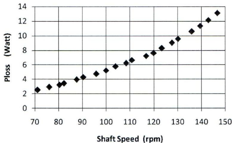
Figure 4. Mechanical power losses and shaft speed
