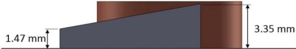
10 Fig. 5. Schematic of the computational domain plate fin and tube heat exchanger with trapezoid winglet pairs (TWPs) of vortex generator.
