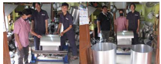
Gbr. 4 Proses pengerolan plat Aluminium
