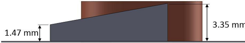
Fig. 5. Schematic of the computational domain plate fin and tube heat exchanger with trapezoid winglet pairs (TWP) of vortex generator.
