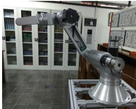
Fig. 2. Developed cast aluminium robotic manipulator
