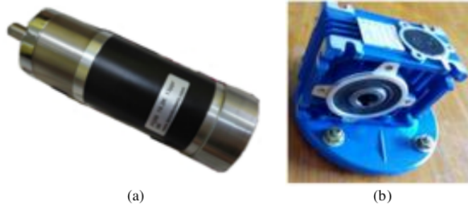
Figure 5. The actuator consists of (a) a PG56 encoder brushed DC motor that is connected to (b) a gearbox with shaft ratio 1:50
