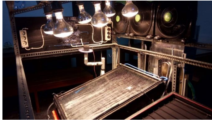
Figure 1. Distillation with fabric and cooler spray
