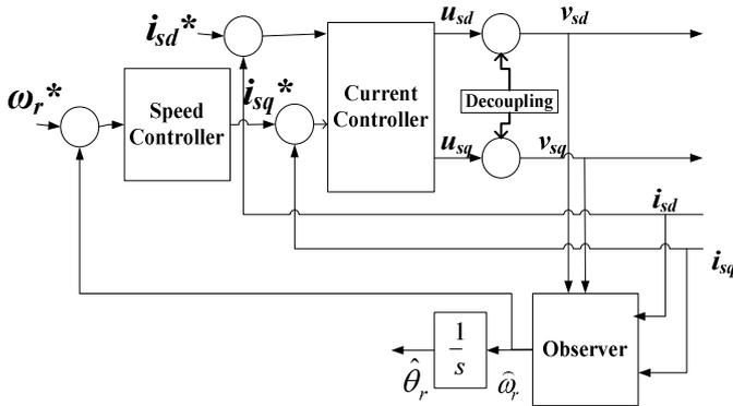
Fig. 1. Block diagram of the sensorless control.
