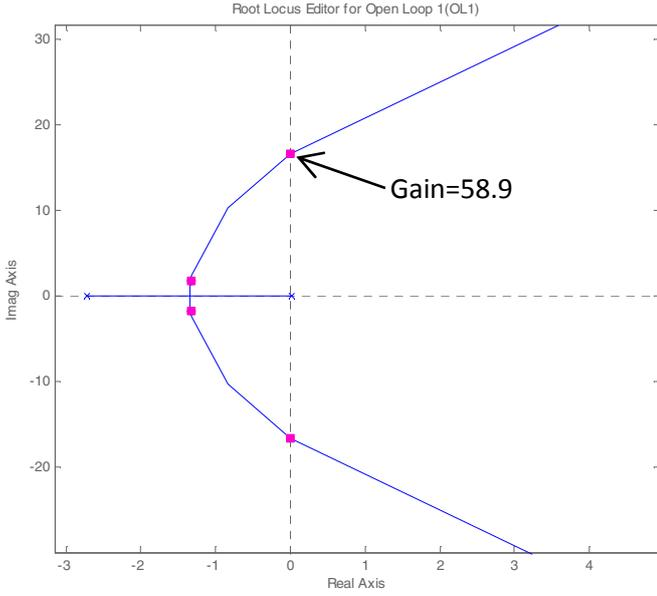
Fig. 10. Root Locus of  $\omega_r^*$  vs  $\omega_r^*$ .
