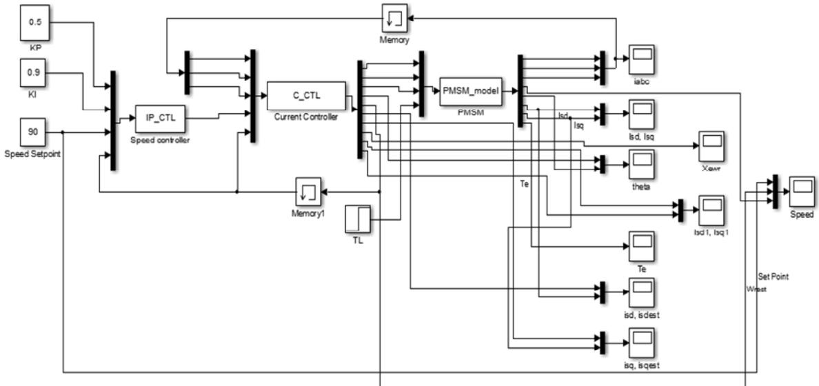
Fig. 2. The Simulink of PMSM sensorless control.
