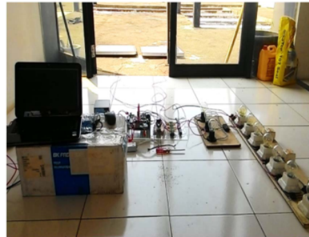
Fig. 3. Solar cell module and boost converter circuit with lamp as a load.
