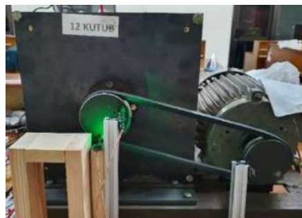
Gambar 9. Generator magnet permanen putaran rendah
